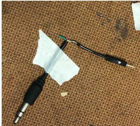
Figure 2-11: Jumper wire soldered onto ground wire of aux cable
