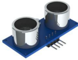
Figure 2-5: Ultrasonic Sensor (Chen, Denzel, 2021)
