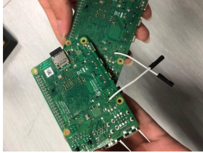
Figure 5-18: Jumper wire soldered onto board
